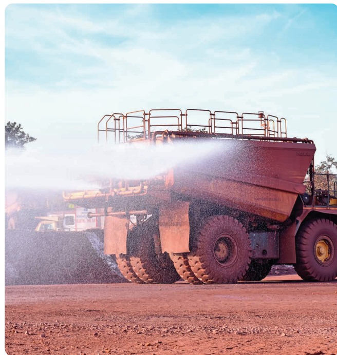
Dust suppression at Noamundi Mine through water sprinkling
